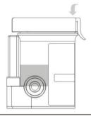
Check cap for tight seal. Technician dates and initials the security seal and places security seal over cap.
