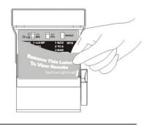
If the test cup includes S.V.T., read adulteration test results between 3 - 5 minutes.
