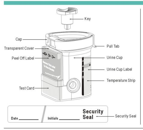
Remove the key by twisting it from the center of the cup cap. Open cap with the Pull Tab. (Key is held by technician.)
